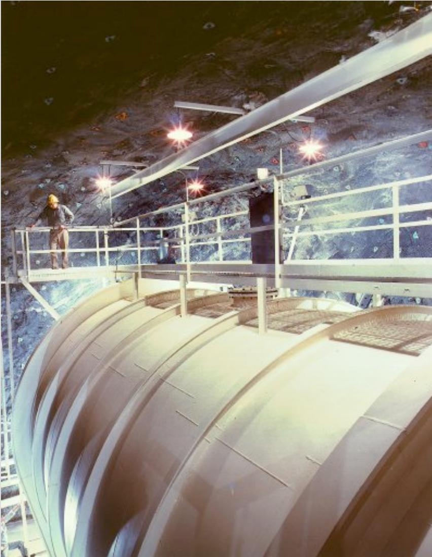
Detector is a large tank containing 600 tons of  $C_2Cl_4$ , situated at 1500m depth in a mine in South Dakota.
