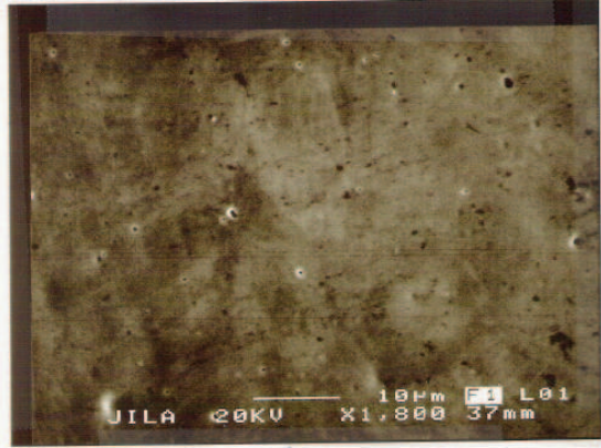
Electro-polished 3 minutes 316 Stainless 1800X
