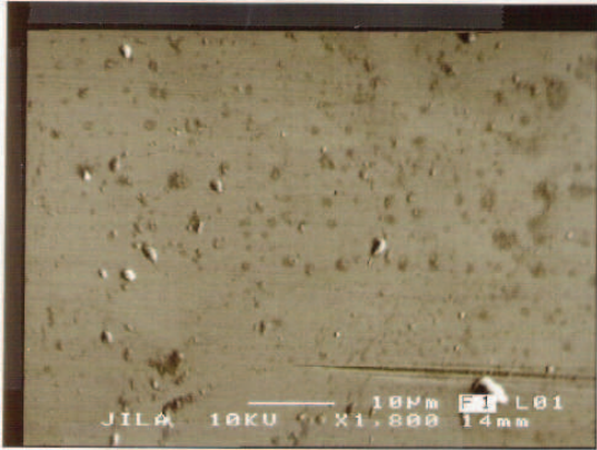
Electro-polished 3 minutes 316 Stainless 70X
