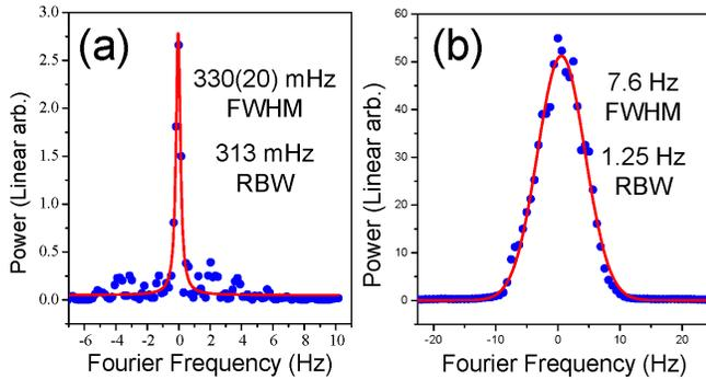
Figure 3. (a) Resolution-bandwidth-limited relative linewidth between the 698-nm probe laser and a narrow 1064-nm reference laser, measured at 1064 nm via a frequency comb, for 3-s averaging time. (b) Identical measurement, taken with a 60-s averaging time
