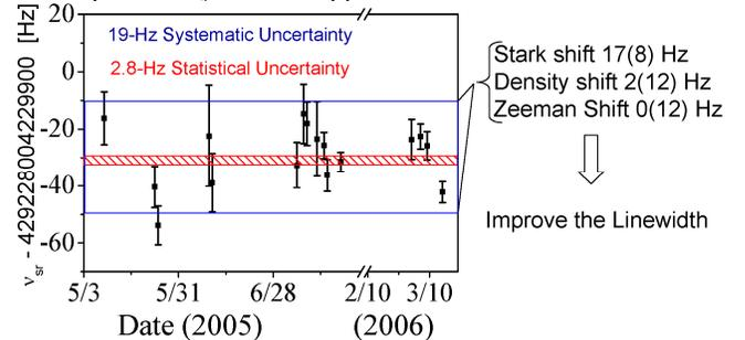
Figure 2. Date record, corrected for systematic effects, of the measured center frequency for the Sr optical lattice clock as reported in [1]. Also included are some preliminary points for additional measurements in 2006. The three most significant sources of systematic uncertainty can be improved by use of a narrower line and with additional averaging.
