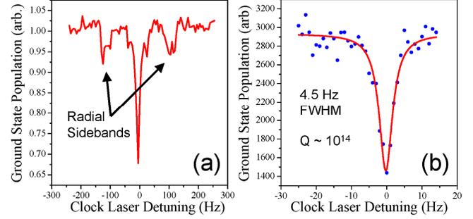
Figure 4. (a) Improvement to the spectroscopic resolution allows the radial sidebands caused by the lattice waist to be measured at  $\sim 120$  Hz offset from the carrier. (b) The clock transition linewidth is now routinely measured to be  $< 5$  Hz.
