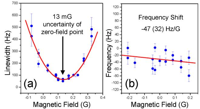
Figure 5. (a) Measurement of the transition linewidth as a function of applied magnetic field along one axis allows calibration of the zero-field point to within an uncertainty of 13 mG. With the improved sub-5-Hz linewidth even more accuracy should be attainable. (b) Simultaneous measurement of the frequency shift with respect to the applied magnetic field then allows the Zeeman shift to be determined with an uncertainty of only  $\sim 1 \times 10^{-15}$ .
