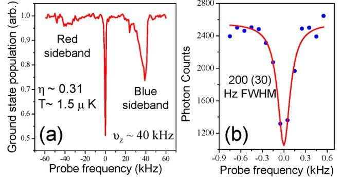
Figure 1. (a) Axial sidebands demonstrating confinement in the Lamb-Dicke regime, and allowing measurement of the sample's temperature. (b) Clock transition, showing the best linewidth used for systematic measurements in 2005 [1].
