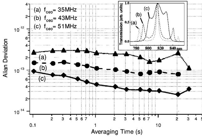
FIG. 3. Allan deviation of beat note at 1064 nm between an iodine-stabilized cw laser and cavity-stabilized fs comb with independent phase locking of  $f_{\text{ceo}}$  to three different values. The inset shows the spectrum of the fs laser transmitted through the reference cavity in each case.
