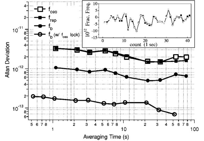
FIG. 2. Measured Allan deviations for the cavity-stabilized fs comb. Open (filled) squares show measurement of  $f_{\text{ceo}}$  ( $f_{\text{rep}}$ ) under case (i). The inset shows a portion of simultaneous counts of fractional frequency fluctuations for  $f_{\text{rep}}$  and  $-f_{\text{ceo}}$ . Circles correspond to measurements of the beat note between the fs comb and an iodine stabilized cw laser at 1064 nm under case (i) (filled) versus case (ii) (open).
