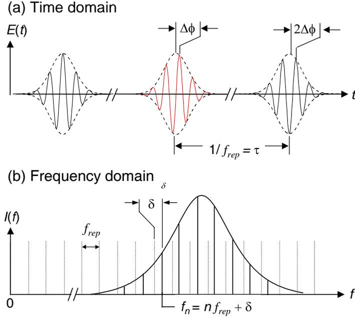
Figure 1 (a) Time-domain picture of the pulses from a modelocked laser and (b) the corresponding frequency comb, where  $\delta$  is the comb frequency offset and  $f_{rep}$  is the comb spacing corresponding to the lasers' repetition rate.
