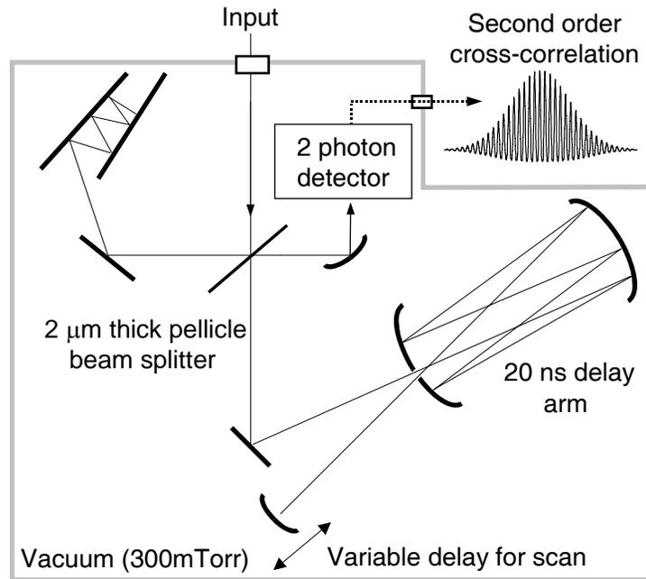
Figure 4 Schematic of the cross-correlator used time domain verification of phase control.
