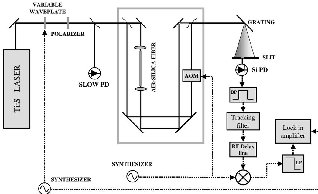
Figure 6 Schematic of the interferometer used to measure the nonlinear phase induced in air-silica microstructure fiber.
