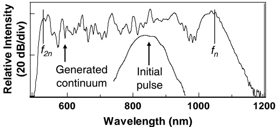
Figure 2 Initial pulse from a KLM Ti:S laser and the output generated by broadening in air-silica microstructure fiber.
