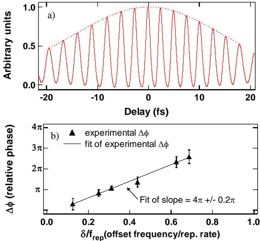
Figure 5 (a) Typical cross-correlation, solid line, and the fit to a Gaussian envelope, dashed line. (b) Experimentally determined values of pulse-to-pulse carrier-envelope phase for different frequency offsets and a linear fit to the results.
