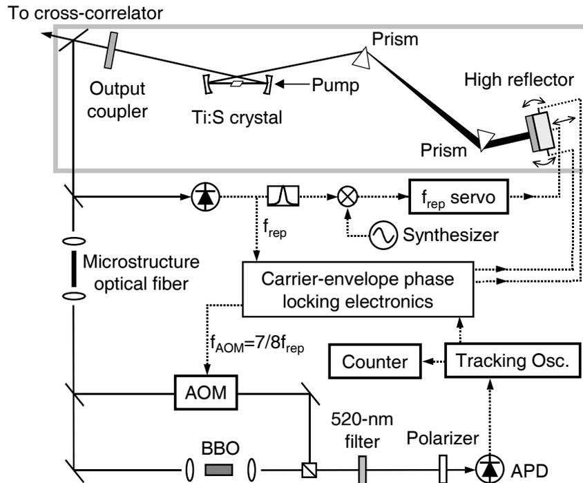
Figure 3 Experimental setup for measuring the absolute position of the femtosecond comb via a self-referencing technique.
