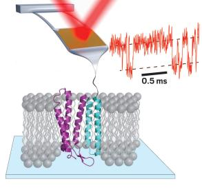
A laser beam (top) detects forces while an AFM cantilever pulls on two bacteriorhodopsin helices (light blue). The SMFS system plots force (vertical axis) versus time as three amino acids reversibly unfold and refold between two intermediate states (dashed lines).
