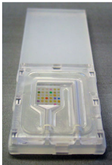
FIGURE 2. A colorimetric sensor uses chemically responsive dyes to detect volatile organic compounds in exhaled breath. Image analysis of the resulting array of color determines the mixture of analytes that was present in the sample. (Courtesy of K. Suslick, University of Illinois–Urbana-Champaign)
