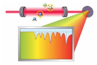
The spectroscopy technique uses many frequencies of laser light to identify trace amounts of atoms and molecules. Each chemical absorbs light at characteristic frequencies, whose pattern forms a signature, or fingerprint, for identifying it.
