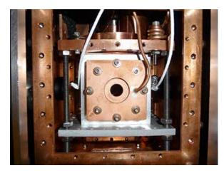
The JILA apparatus couples a mid-infrared frequency comb to an optical cavity containing a buffer gas chamber, in which samples are cooled to near absolute zero. "Calming down" the sample molecules by molecular cooling results in a cleaner, more rapidly interpreted "molecular fingerprint" in the frequency-comb spectra. [Image: Spaun/JILA]
