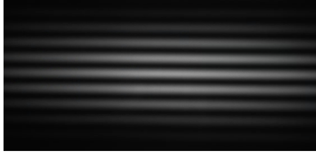
Figure 6.11: The fringes of the accordion lattice, here at a relatively large spacing, are imaged onto a camera.
