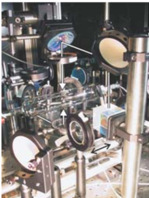
Fig. 8. Picture of the vertical-beam optics for the MOT omitted from Fig. 7. Figure shows the location of the track (black arrow) and the vertical MOT beams (white arrows). The coils of the MOT/quadropole trap are translated left, towards the science cell, out of the field of view of this photograph.
