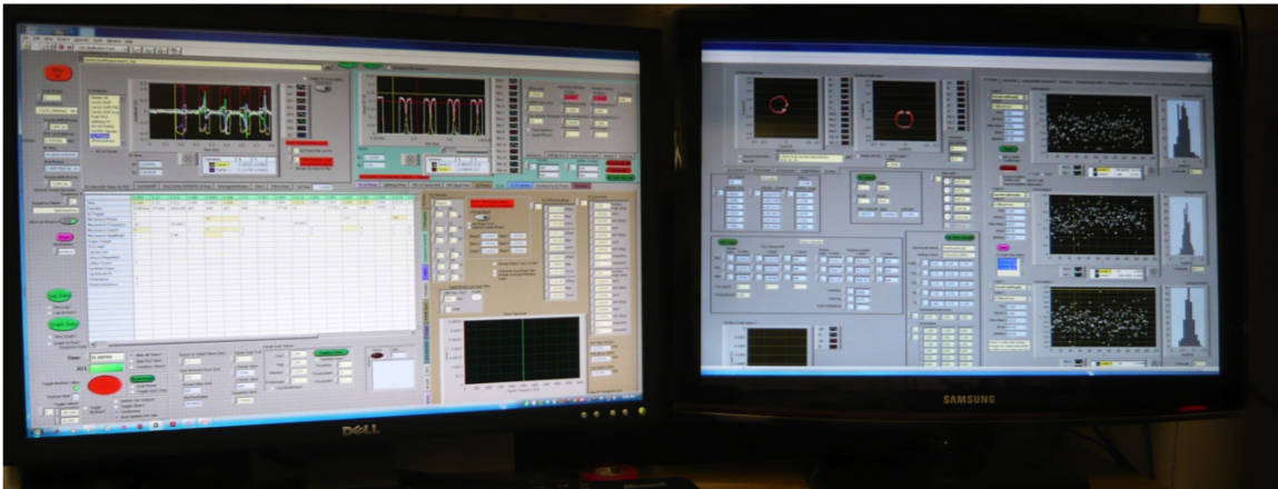
Figure 5.6: Screenshot of data acquisition program showing experimental control sequence table (left monitor, middle), raw data (left monitor, top), real-time fitting of the IQ signals in the complex plane (right monitor, left top) and accumulation of measurement statistics from different experimental trials (right monitor, right panel).
