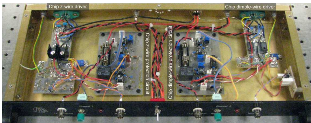
Figure 4.14: (Color) The chip driver and protection box. The outer two circuits are the two (main Z and dimple) chip driver circuits with the power op-amp mounted on the rear of the box for passive cooling and heat sinking. The inner two circuits are the two protection circuits. Both circuits are described in detail in Appendix A.
