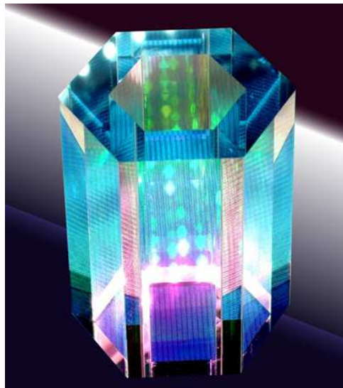
Figure 3.20: (Color) Photo of the AQuA cell hexagonal cell after polishing and AR coating.
