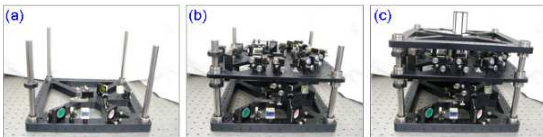
Figure 5.19: (Color) Photo of the AQUA cell optomechanics package, view from the side showing the tiers. (a) Bottom tier with push beam optics, and the input dipole beam optics. The four steel rails are mounted to roller bearing sleeves that are press-fit into the base plate. (b) Second tier has the 2D^+ MOT optics on the bottom side, and the MM MOT optics on the top side. The second tier also has roller bearings press-fit into it to allow it to be positioned vertically. The second tier is held in place against gravity temporarily by a split-ring clamp attached to the steel rods. (c) The third tier holds the AQUA cell. Alignment in all three axes is done with ball bearing grooves in the plate and clamps. The top of the third tier is left empty to incorporate the quantum computing optics around the Hex cell.
