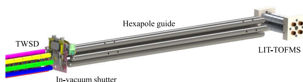
FIG. 1. Simplified rendering of the proposed, combined apparatus. Following the TWSD is an in-vacuum molecular beam shutter. The decelerated beam admitted through the shutter is guided by a hexapole and focused into the ion trap.
