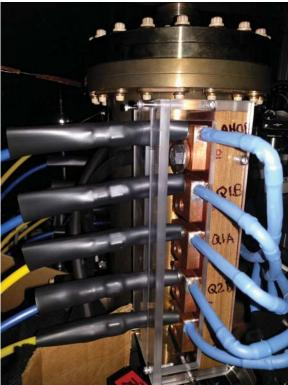
Figure 2.29: Left: CAD model of the water and electrical hookups for the top bucket coils. Right: Photo of the connections on the mounting tabs on main chamber.
