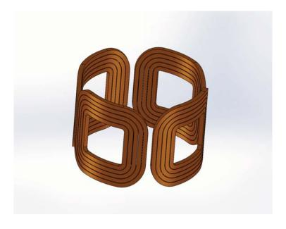
Figure 2.14: CAD model showing one set of quadrant coils. The two sets of quadrant coils are placed inside the bucket windows, on opposite sides of the atoms.
