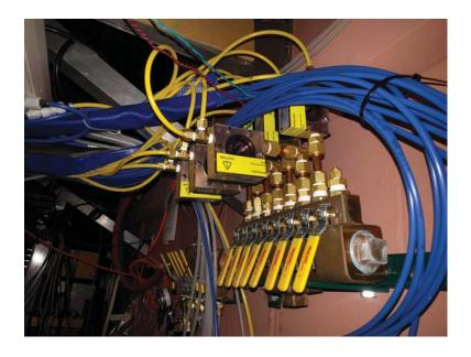
Figure 2.31: Photo of part of the water cooling manifold, with flowmeters shown.
