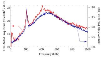
Fig. 2. (Color online) Comparison of the intensity noise spectrum with the frequency noise of a comb tooth near the optical carrier for  $I \approx 1.1 I_{\rm th}$ .
