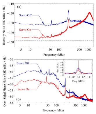
Fig. 3. (Color online) (a) Intensity noise spectrum of the oscillator with and without the servo action. The dashed line indicates the shot-noise floor. (b) Reduction in the phase noise near the carrier frequency due to the servo (inset: rf spectrum of the phase-locked optical beatnote).
