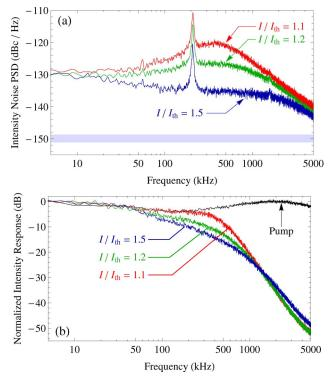
Fig. 1. (Color online) (a) Intensity noise spectrum of the Yb oscillator at various pump powers normalized to DC signal. The shaded box indicates the shot-noise floor of the measurements. (b) Intensity modulation transfer functions for the oscillator and the pump diode.
