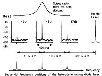
Fig. 4. Filter-cavity mechanism showing its sideband se-
