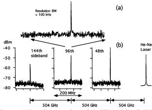
Fig. 3. (a) Beat between the 96th (1-THz) sideband of the He–Ne laser and the diode laser. (b) Beats between the 48th (505-GHz), 96th, and 144th (1.515-THz) sidebands and the diode laser. Incident power, 150  $\mu$ W.
