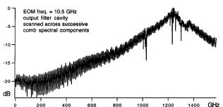
Fig. 2. OFC generator output spectrum as the filter-cavity resonance is scanned through the comb spectrum. The comb-line spacing is 10.5 GHz. The adjacent order of the filter cavity leads to overlapping spectra below ~200 GHz.
