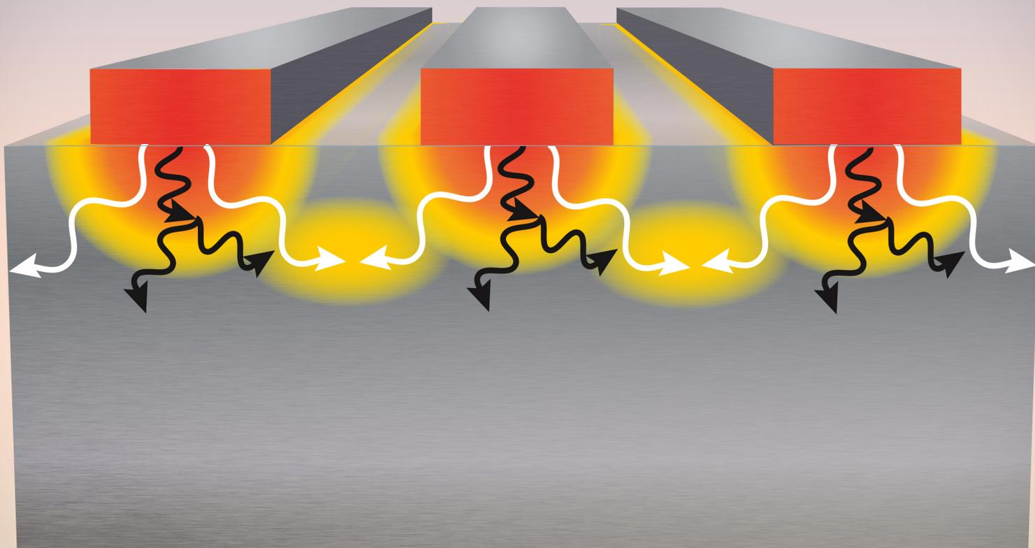
When closely spaced heated nickel nanowires emit lattice vibrations known as phonons into underlying materials, the phonons efficiently collide and transport heat away. This discovery has immediate application to the design of integrated circuits, nanoenhanced solar cells, and other electronics employing nanostructures. Credit: K. Hooeboom-Pot and the Kapteyn/Murnane group, JILA
