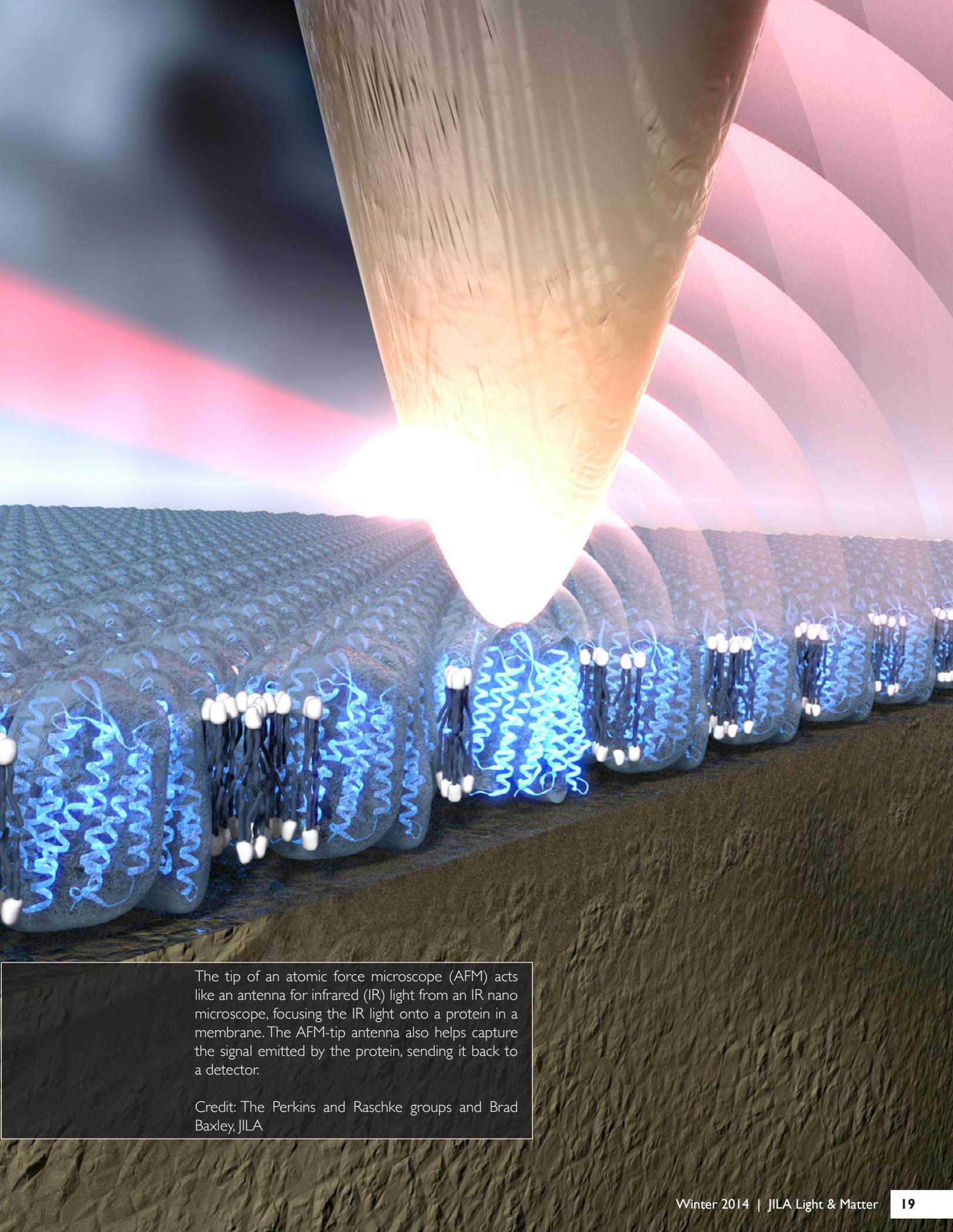
The tip of an atomic force microscope (AFM) acts like an antenna for infrared (IR) light from an IR nano microscope, focusing the IR light onto a protein in a membrane. The AFM-tip antenna also helps capture the signal emitted by the protein, sending it back to a detector.
