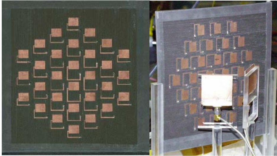
Figure 3.4. Photographs of both sides of a 30-element X-band two-layer quasi-optical lens antenna array with patch antenna elements. The one on the right also shows the ground planes of the receiving antennas placed on the focal arc of the lens array.
