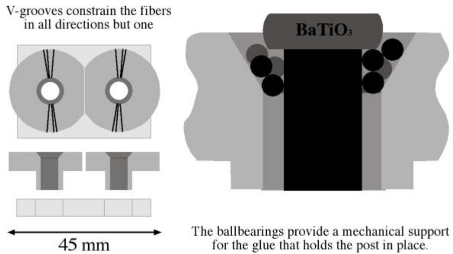
Figure 7.2 Mechanical mount for the first version of the autotuning filter with spherical photorefractive crystals
