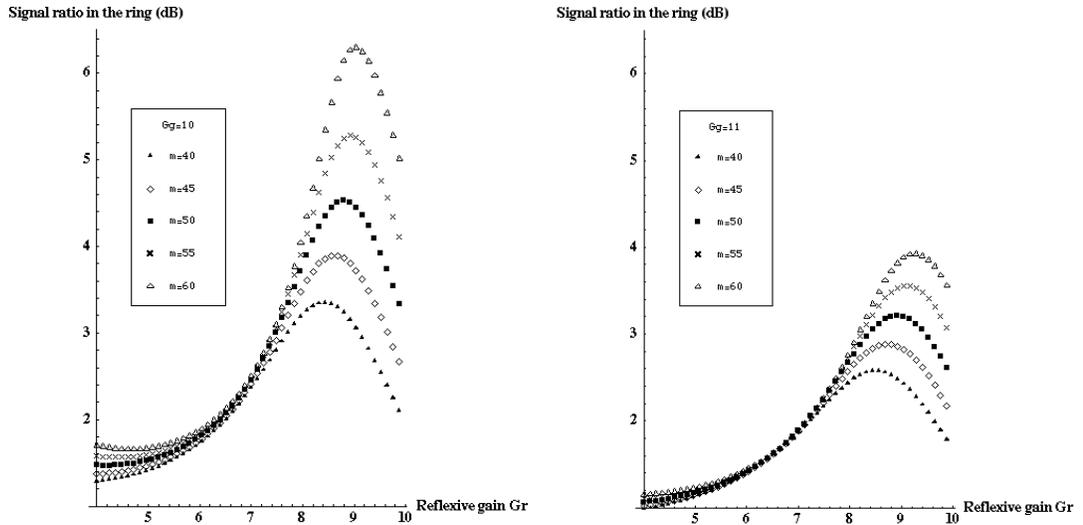
Figure 2.21. Left side:  $S_1/S_2$  vs.  $Gr$  for  $m=60, 55, 50, 45,$  and  $40$  from top to bottom with  $T=0.5, Gg=10,$  and  $P_1/P_2=0.2$  dB. Right side: same values except  $Gg=11$ .
