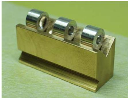
Figure 3.14: 3 lens subsystem. The lenses are placed in cylindrical mounts that have the exact same outer diameter to keep the lenses centered relative to each other. The v-groove allows only one translation.
