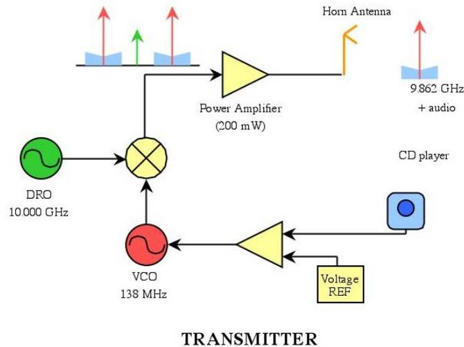
Figure 3.3. Diagram of the circuit that drives the horn antennas.
