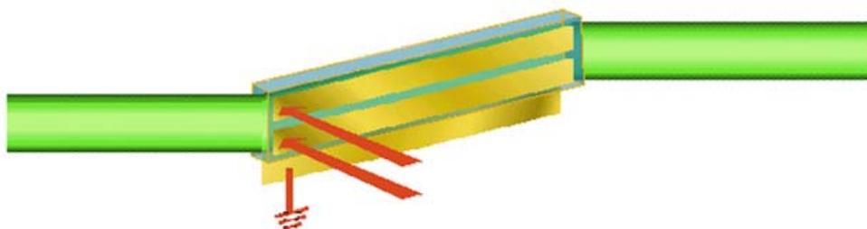
Figure 3.8. Electro-optic modulation: a channelized electro-optic modulator made from magnesium doped lithium niobate crystal ( $\text{Mg}:\text{LiNbO}_3$ ) imposes spatial and temporal modulation on the optical carrier.
