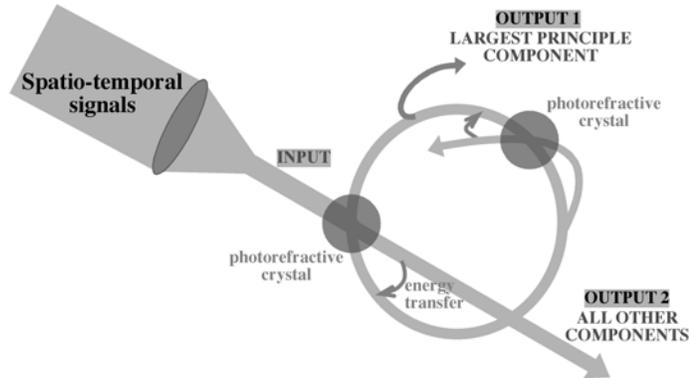
Figure 1.1. Schematic diagram of the autotuning filter.
