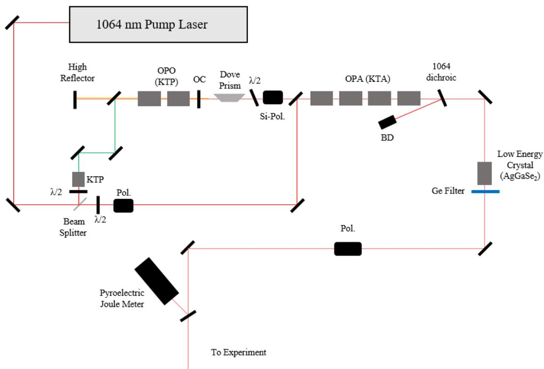
Figure 2.4. Schematic of the Optical Parametric Oscillator/Amplifier system ( $\lambda/2$ , half-wave plate; OC, output coupler; BD, beam dump; Si-Pol., silicon polarizer; Pol., polarizer).
