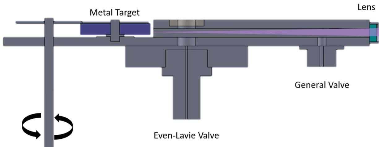
Figure 2.1. Schematic of the ion source. In the laser vaporization method, a laser propagates from right to left and is focused onto the edge of a metal target (see text). In the entrainment of volatile gases experiment, the target gas is introduced with a general valve and entrained into the main expansion (see text), additionally ions can be produced using only the main expansion.
