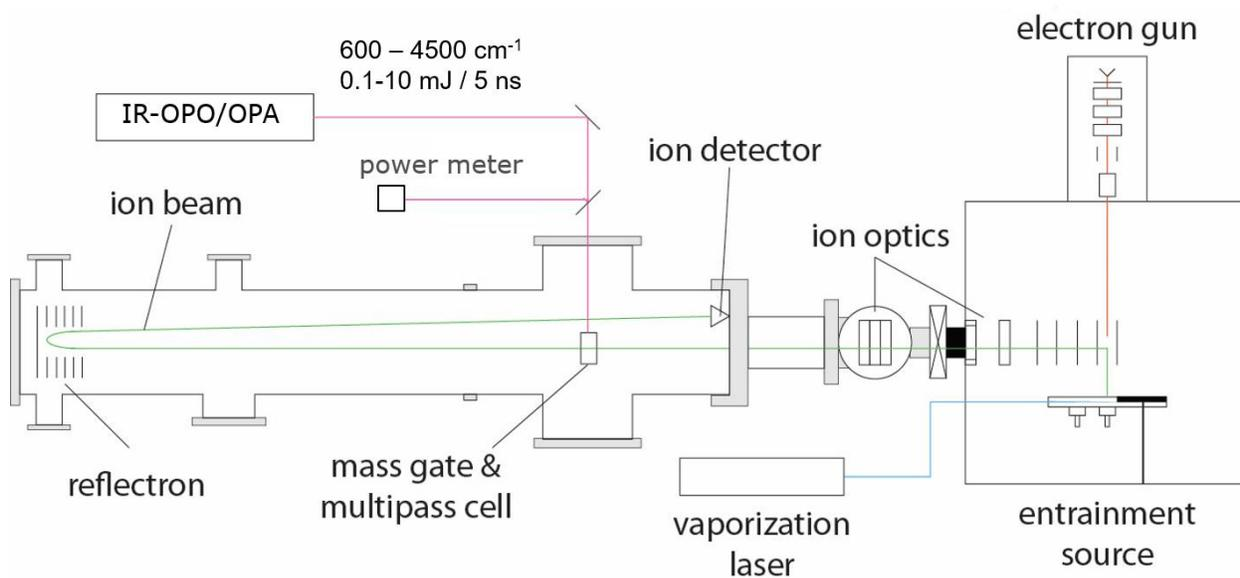
Figure 2.2. Diagram of the experimental apparatus with paths outlined of the vaporization laser (blue), ion path (green), electron beam (red), and laser (purple).
