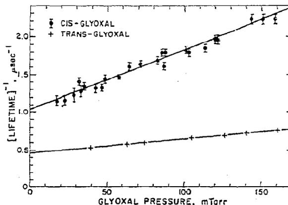
Fig. 2.  $(\text{Lifetime})^{-1}$  as a function of glyoxal pressure for *cis*- and *trans*-glyoxal fluorescence. In each case excitation is near the 0-0 band with the observed fluorescence being primarily the  $8^0_0$  band.
