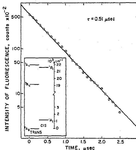
Fig. 1. Typical decay curve for the sum of 6000 pulses. The laser is exciting the *cis*-glyoxal 0-0 band. The fluorescence is primarily the  $8^0_0$  band at a pressure of about 127 mtorr of glyoxal. Inset is a diagram of the five levels observed for glyoxal.
