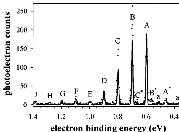
FIG. 1. 364 nm photoelectron spectrum of  $\text{SnO}^-$  taken at 180 K (dotted line) and Franck–Condon simulation (solid line).
