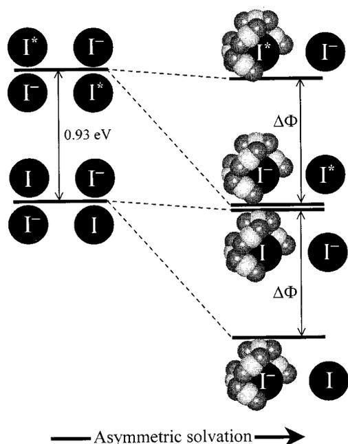
FIG. 10. An energy diagram illustrating the mechanism of spin-orbit relaxation by solvent mediated electron transfer from  $I^-$  to  $I^*$  in an asymmetrically solvated cluster. The required resonance between the  $X \cdot I^- \cdots I^*$  and  $X \cdot I^- \cdots I^-$  electronic states occurs when the differential solvation energy ( $\Delta\Phi$ ) is equal to the spin-orbit energy gap in iodine (0.93 eV).
