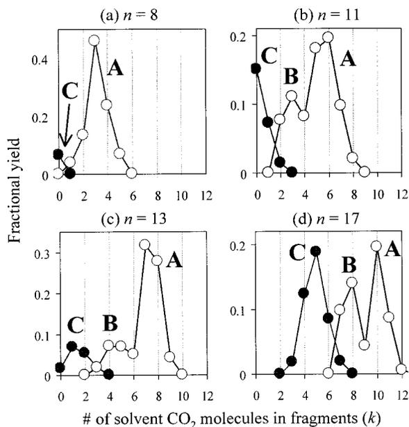
FIG. 5. Photofragment ion distributions in 395 nm photodissociation of  $I_2^-(CO_2)_n$  with  $n=(a) 8, (b) 11, (c) 13,$  and  $(d) 17$ . The fractional fragment populations are obtained by integrating the corresponding peaks in fragment mass spectra. Filled circles indicate caged  $I_2^-(CO_2)_k$  products, open circles correspond to uncaged  $I^-(CO_2)_k$  fragments. A, B, and C label the corresponding reaction channels, as defined in Sec. I.
