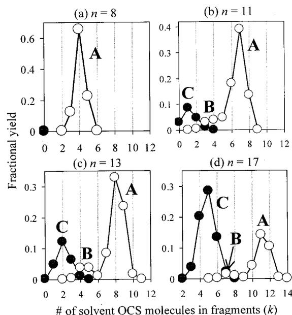
FIG. 6. Photofragment ion distributions in 395 nm photodissociation of  $I_2^-(OCS)_n$  with  $n=(a) 8, (b) 11, (c) 13,$  and  $(d) 17$ . The fractional fragment populations are obtained by integrating the corresponding peaks in fragment mass spectra. Filled circles indicate caged  $I_2^-(OCS)_k$  products, open circles correspond to uncaged  $I^-(OCS)_k$  fragments. A, B, and C label the corresponding reaction channels, as defined in Sec. I.
