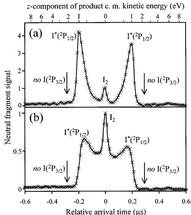
FIG. 3. Neutral photofragment TOF spectra obtained in 395 nm photodestruction of  $I_2^-$  with the laser polarization (a) parallel and (b) perpendicular to the flight axis ( $z$ ). The fragment spatial distributions are truncated at the entrance into the reflectron (see Fig. 2). Top axis is the  $z$ -component of fragment c.m. translational energy.
