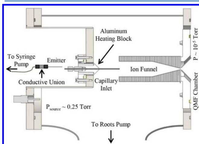
Figure 1. Electrospray ion source for the SIFT.
