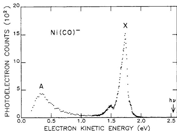
**Figure 1.** Photoelectron spectrum of  $\text{Ni}(\text{CO})_1^-$  obtained with 2.540-eV photons; ion current was about 18 pA. Peak X corresponds to the transition to ground-state  $\text{Ni}(\text{CO})$  which defines the electron affinity.
