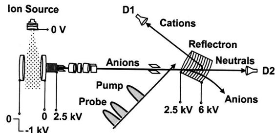
FIG. 1. Schematic diagram of the ion-beam part of the photodetachment-photoionization apparatus.
