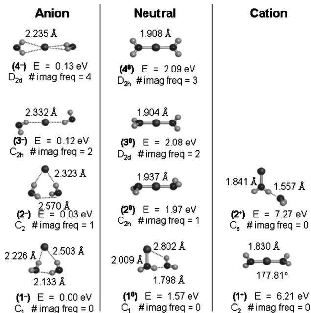
FIG. 6.  $\text{Cu}(\text{H}_2\text{O})_2$  anion, neutral, and cation stationary points optimized at the MP2(fc)/(aug-SDB aug-cc-pVTZ) level of theory. Electronic energy differences are calculated from the global minimum of the anion surface, at the CCSD(T)/(aug-SDB aug-cc-pVDZ) level of theory.
