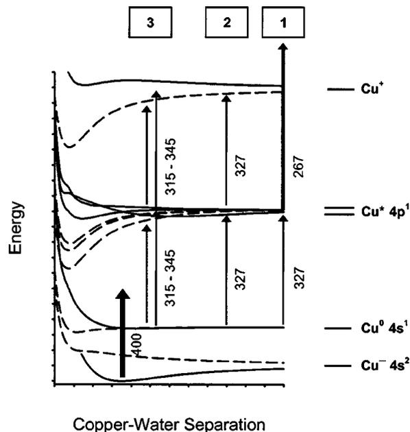
FIG. 2. Schematic representation of the measurements performed, superimposed on schematic  $\text{Cu}(\text{H}_2\text{O})_2$  anion, neutral, excited state, and cation potential energy curves. The figure is adapted from Refs. 13 and 23. Probe schemes 1–3 are discussed in the text.
