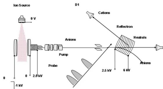
FIG. 2. Schematic diagram of the ion beam portion of the photodetachment-photoionization apparatus.
