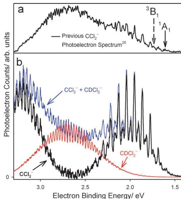
**Fig. 1**  $\text{CCl}_2^-$  magic-angle photoelectron spectra. (a) The 364 nm  $\text{CCl}_2^-$  spectrum from the previous study.<sup>26</sup> (b) The new 351 nm spectrum collected at  $m/z \approx 81$  minimizes the  $\text{CDCl}_2^-$  contamination. The pure  $\text{CDCl}_2^-$  spectrum is scaled and subtracted from the  $m/z \approx 81$  trace to yield the “clean”  $\text{CCl}_2^-$  spectrum.
