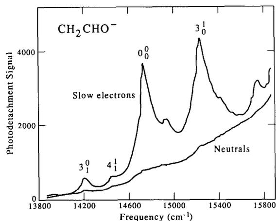
Fig. 1. Photodetachment cross section of  $\text{CH}_2\text{CHO}^-$  taken with  $1 \text{ cm}^{-1}$  resolution (from ref. [12]) where  $\nu_3$  is the CCO bend and  $\nu_4$  is the torsional mode. The  $3_1^0$  bending hot band is investigated under high resolution in this study.
