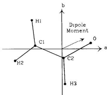
Fig. 3. Structure, principal axes, and dipole moment of the ground vibrationless state of acetaldehyde enolate anion, as determined in ref. [12]. Excitation of  $\nu=1$  in the CCO bend results in substantial opening of the CCO bond angle from  $129^\circ$  to  $136^\circ$ .
