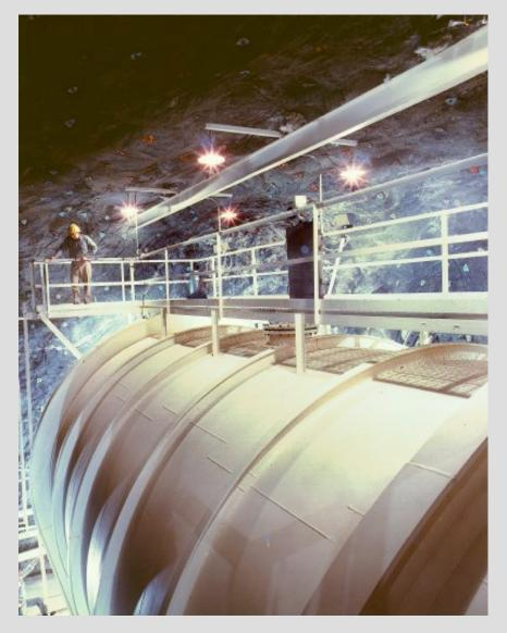
Detector is a large tank containing 600 tons of  $C_2CI_4$ , situated at 1500m depth in a mine in South Dakota.
