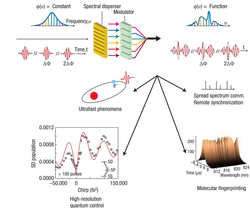
**Figure 1** A schematic of an OAWG showing its applications. The OAWG needs to maintain optical phase coherence and requires a massive amount of parallel processing of spectral phase and amplitude. The technology will have a profound impact on a range of important applications. ( $\nu$ : frequency,  $t$ : time;  $\Delta\Phi$ : pulse-to-pulse carrier-envelope phase offset;  $\phi(\nu)$ : pulse spectral phase)
