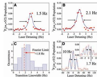
a 20.8(3)-Hz period and 10.4(2)-Hz fringe width, with data shown as open circles. Inset shows a Ramsey pattern with a 1.7(1)-Hz fringe FWHM.
