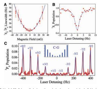
residual Stark shifts. (**C**) A field of 0.77 G is applied along the polarization axis, and the individual Fourier-limited (10 Hz)  $\pi$  transitions are easily resolved. Data are shown in red, and a fit of 10 evenly spaced transitions is shown in blue. The calculated transition probabilities based on Clebsch-Gordan (C-G) coefficients are included in the inset. In (B) and (C), the population is scaled by the total number of atoms available for spectroscopy (~10<sup>4</sup>).
