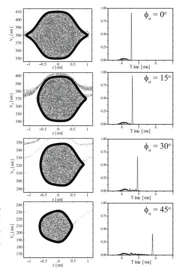
**Fig. 12.** The left column is stable phase space of molecules decelerated inside the QGD. The solid line is the separatrix predicted by the theory, while the points represent positions of molecule in the 3D Monte Carlo simulations. The right column shows the ToF spectra of OH molecules in the  $|2\pm 2,-\rangle$  state at the exit of this decelerator which has 142 deceleration stages, along with 142 quadrupole stages.
