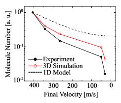
Fig. 2. (Color online) Experimental (dots) and Monte Carlo simulation (open circles) results for total molecule number as a function of final velocity. The dashed curve is the expected decelerator efficiency calculated from the one-dimensional (1D) theoretical model of reference [20].
