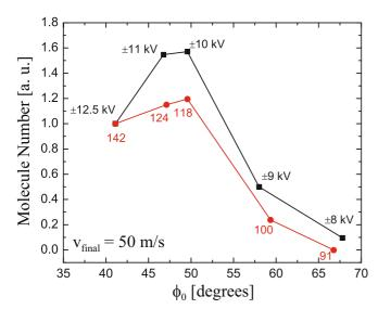
**Fig. 4.** (Color online) Experimental results from changing the voltage on decelerator rods (squares) and decreasing the effective decelerator length (circles). Effective slower length is modified by initially operating the decelerator at  $\phi_0=0^\circ$ , S=3, then slowing with S=1 to  $v_{final}=50$  m/s for the number of stages labeled. Both curves illustrate that transverse/longitudinal couplings are strongly dependent on phase angle, and have a marked effect on decelerator efficiency.
