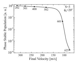
Fig. 7. Monte Carlo results for decelerated molecule number using S=3 and  $\phi_0=20^{\circ}$  versus final velocity. The number next to each data point is the number of stages used. Because of transverse overfocusing and longitudinal velocity filtering, essentially no molecules survive below 100 m/s.
