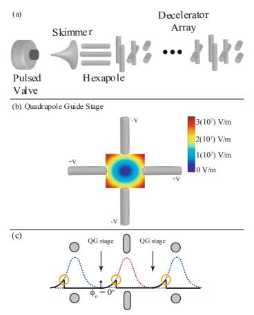
Fig. 10. (Color online) Quadrupole-guiding decelerator. (a) Schematic of QGD. (b) Electric field of quadrupole guiding stage energized to  $\pm 12.5$  kV. (c) Switching scheme for deceleration with the QGD.
