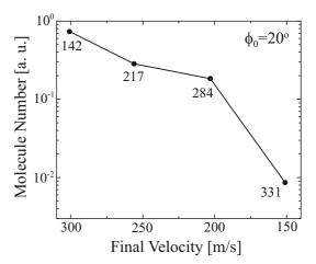
**Fig. 9.** Monte Carlo results of decelerated molecule number using S=3+ and  $\phi_0=20^{\circ}$  versus final velocity. The number next to each data point is the number of stages used. Because of transverse overfocusing, essentially no molecules survive below 100 m/s.
