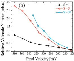
Fig. 8. (Color online) (a) Experimental ToF data of decelerated OH packets produced using the S=3+ modified overtone. Also shown for comparison is the experimental bunching packet for operation at S=1. (b) The de-convolved, integrated molecule number calculated from S=3+ (open squares), S=3 (open circles), and S=1 (dots) data.
