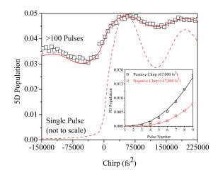
FIG. 4 (color online). The  $5D_{5/2} F = 4$  excited state fluorescence is measured (squares) under steady-state excitation (>100 pulses) vs the applied linear frequency chirp. The solid line indicates the steady-state theory and the dashed line is the single-pulse theory. Inset: the signal (symbols) vs pulse number for two values of equal and opposite chirp; the solid and dashed lines are theoretical predictions.
