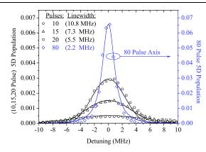
FIG. 3 (color online). The  $5D_{5/2}$  F = 4 line shape is measured (symbols) vs the number of applied femtosecond pulses (10, 15, 20, 80 pulses) with the corresponding FWHM linewidth in the legend. The Lorenztian linewidth of 2.2 MHz after 80 pulses is the asymptotic power-broadened linewidth.
