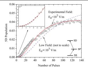
FIG. 2 (color online). The on-resonance  $5D_{5/2} F = 4$  fluorescence signal is measured (squares) at a field strength of  $E_o = 10^7 \text{ V/m}$  vs the number of pulses. The solid (dashed) line is the theoretically predicted excited state populations under experimental (asymptotically low) field strengths. The inset shows the quadratic scaling for the first 15 pulses.
