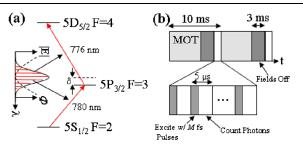
FIG. 1 (color online). (a) Simplified energy level diagram of the three relevant atomic states and frequency domain representation of the chirped comb.  $\delta$  is the detuning of the intermediate state from half the two-photon transition frequency. (b) Timing diagram used in the experiments.
