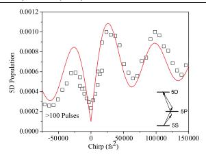
FIG. 5 (color online). Measured fluorescence (squares) and theoretical prediction (solid line) for the case of destructive quantum interference vs linear frequency chirp. The inset shows two of the many two-photon resonant comb mode pairs symmetrically detuned from the intermediate  $5P_{3/2}$  F = 3 resonance; the closest pair is  $\pm 50$  MHz ( $\pm f_r/2$ ) detuned.
