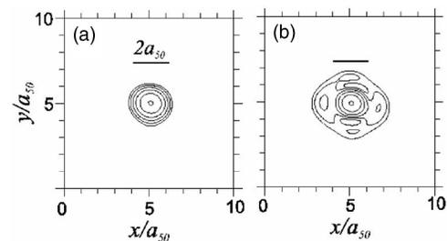
FIG. 4. Results of numerical calculations for the fluence distribution in the focal area using an  $f=500$  mm lens (without pipe) at (a) 50  $\mu$ J and (b) 600  $\mu$ J. The lowest contour value is 0.03 of the maximum contour value in all panels. The interval between the contours changes as  $2^n$ , where  $n$  is the contour number. Horizontal scale indicates the diameter  $2a_{50}$  of the fluence distribution obtained at 50  $\mu$ J at the  $1/e^2$  level.
