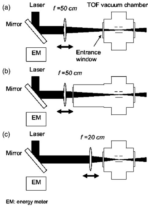
FIG. 1. Experimental setups. The length of the focusing lens and the position of the entrance window with respect to the lens are changed in order to vary the strength of the self-action effects in the window. (a)  $f=500$  mm, large distance between lens and window (strong self-action effects), (b)  $f=500$  mm, small distance between lens and window (small self-action effects), and (c)  $f=200$  mm, short distance between lens and window (small self-action effects).
