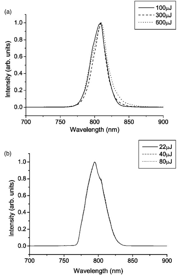
FIG. 2. Pulse spectra at different input energies, obtained using the  $f=500$  mm lens, (a) without pipe. (b) Same, but for the  $f=200$  mm lens. Note that in panel (b), the different curves coincide.
